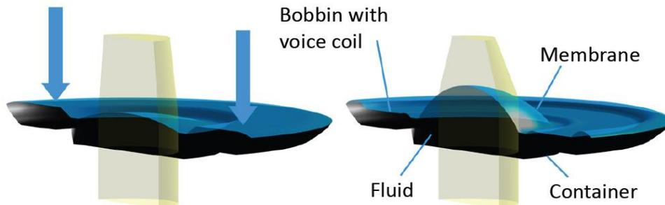
Figure 4: Working principle of the sealed lens container filled with an optical fluid and embedded in an EL-12-30-TC housing.
