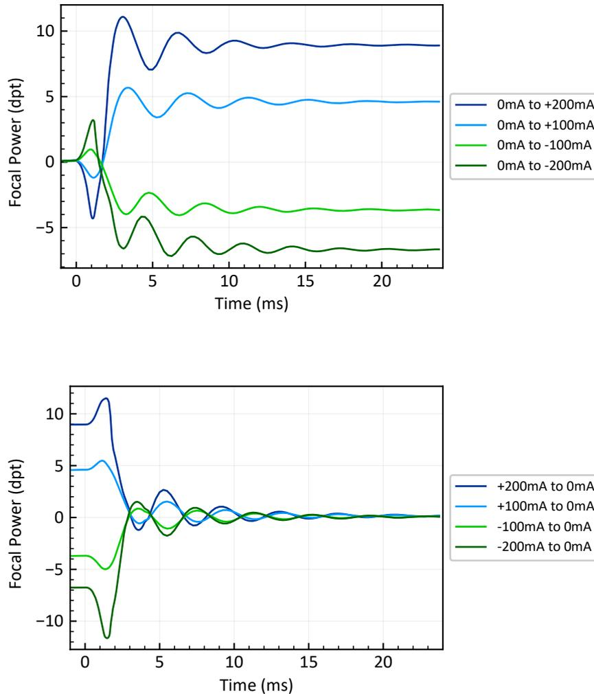
Figure 9: Typical focal power response of the EL-12-30-TC for several current steps. The upper plot shows a series of steps from low to high current and the lower plot for steps from high to low current.
