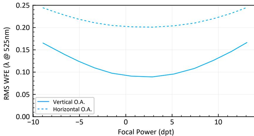
Figure 7: Typical wavefront error of the EL-12-30-TC vs focal power with optical axis vertical and horizontal (@525nm, measured over 80% of the clear aperture).
