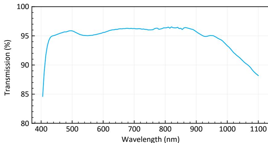
Figure 6: Transmission spectrum of standard EL-12-30-TC.
